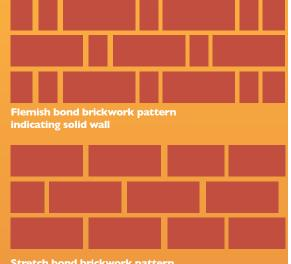
Stretch bond brickwork pattern indicating a cavity wall
